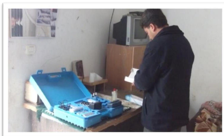
Figure 14: Residual Chlorine Testing Equipment
